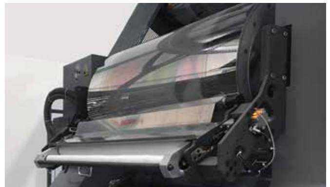
FilmCylinderCleaning installation in a film extrusion production line.
