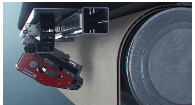
Automatic Breakaway design of cleaning head keeps it safe from damages.
