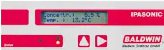
*Digital display of currently measured alcohol and temperature values on BALDWIN desk units*
