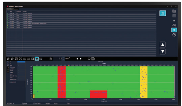
Defender Waste Manager can interface to rewinding, slitting, and sheeting equipment to automatically control when they stop/reject—allowing for fast and easy removal of defective material.
